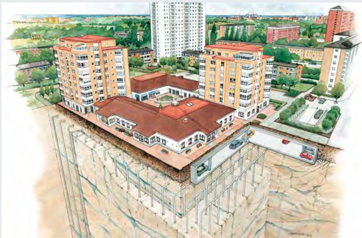
Figure 1. Borehole thermal energy storage. Source: Geotec, Sweden.
