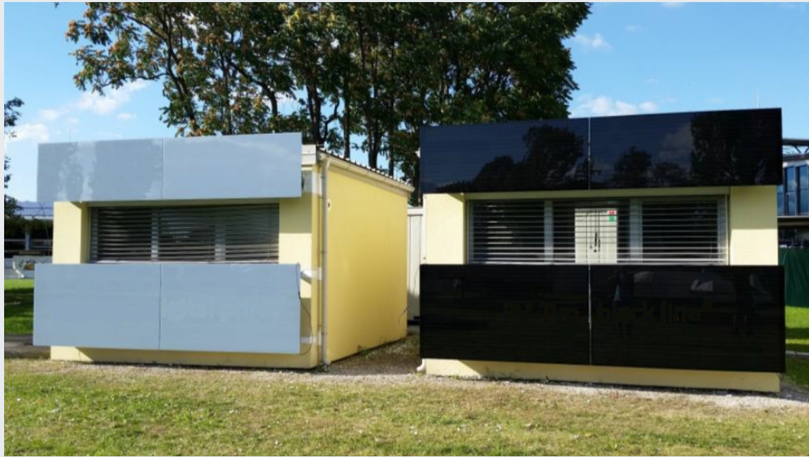
Fig. 1: Test boxes including a façade-integrated heat pump prototype for cooling. Two types of PV are tested at Graz Technical University campus.
