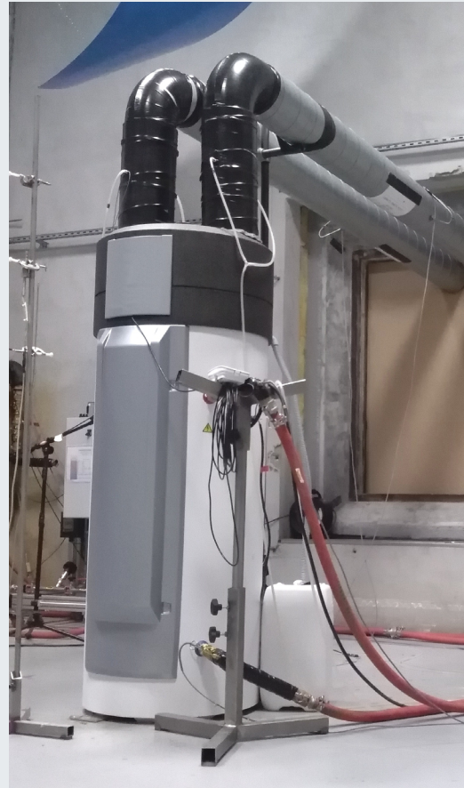
Fig. 1: Exhaust Air Heat Pump Water Heater unit installed in CETIAT's double reverberant room. [Source: CETIAT, France]
