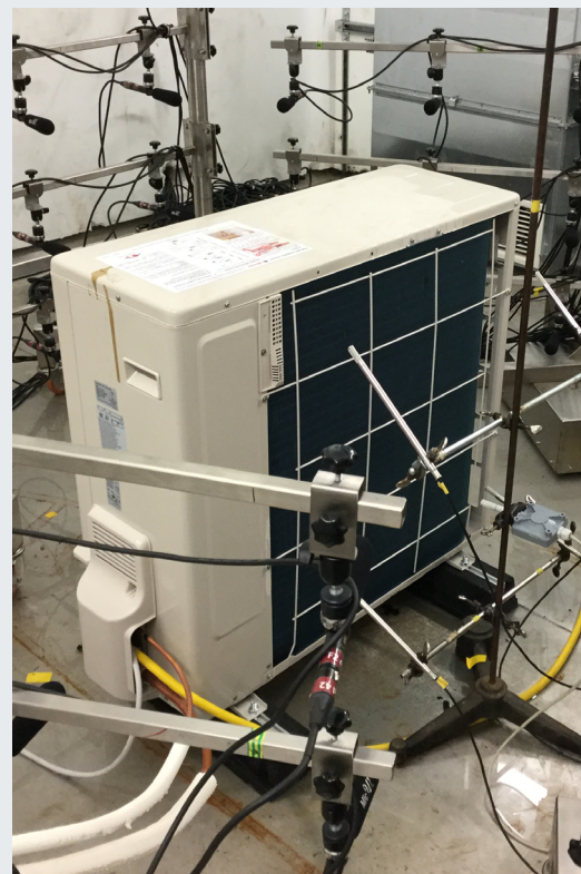
Fig. 2: Air-to-Water Heat Pump surrounded by the acoustic dome with more than 60 microphones installed in the climate chamber of AIT. [Source: AIT, Austria]
